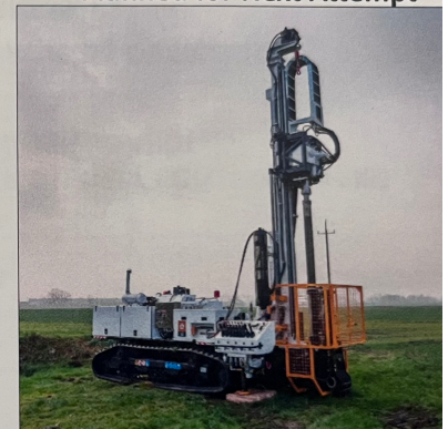
Big Rig - Sonic Drill Rig Planned for Next Attempt
