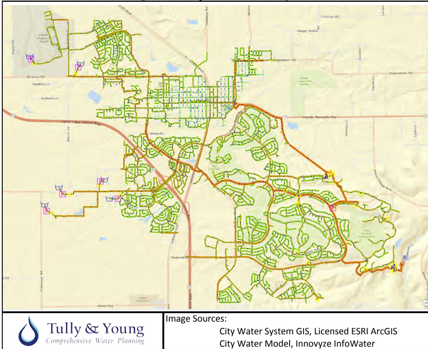
As shown in **Figure 3-5**, the City’s infrastructure is depicted down to the individual street level. This level of detail is further refined with data input recognizing the physical details of each pipe in the system (diameter and length) as well as the age of each pipe in the system.<sup>3</sup> The information related to the water system model in terms of pipe diameter, length, and ages is more fully developed in **Chapter 9**.
