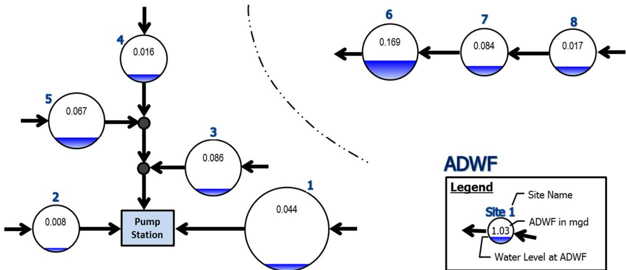
Figure 4-1. Dry Weather Flow Schematic
