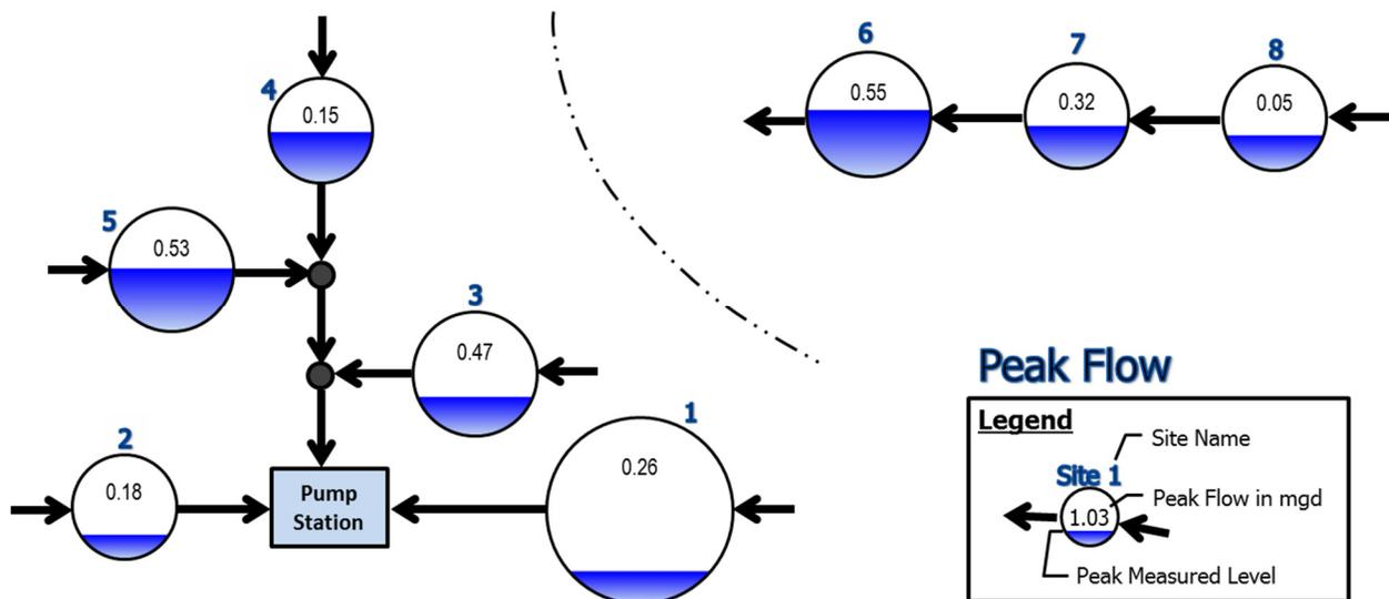
Figure ES-2. Wet Weather Flow Schematic
