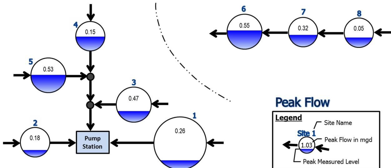
Figure 4-2. Wet Weather Flow Schematic
