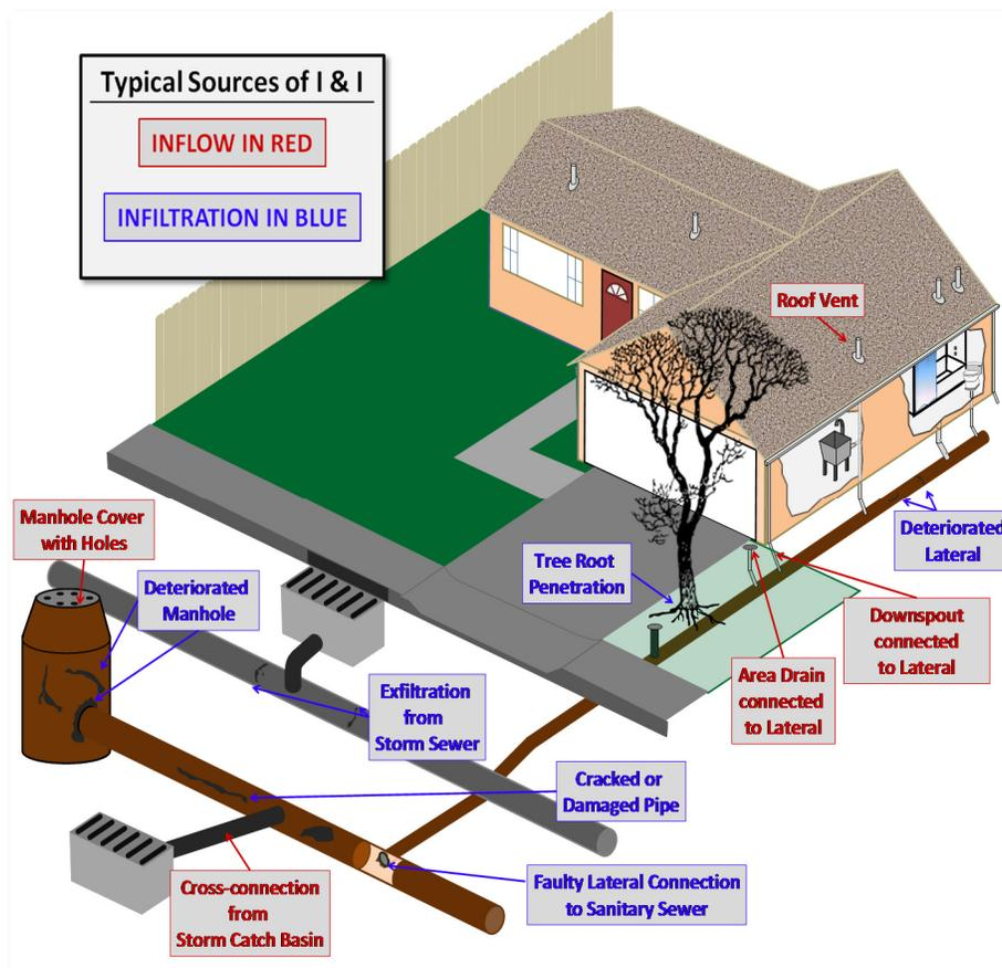
Figure 2-4. Typical Sources of Infiltration and Inflow
