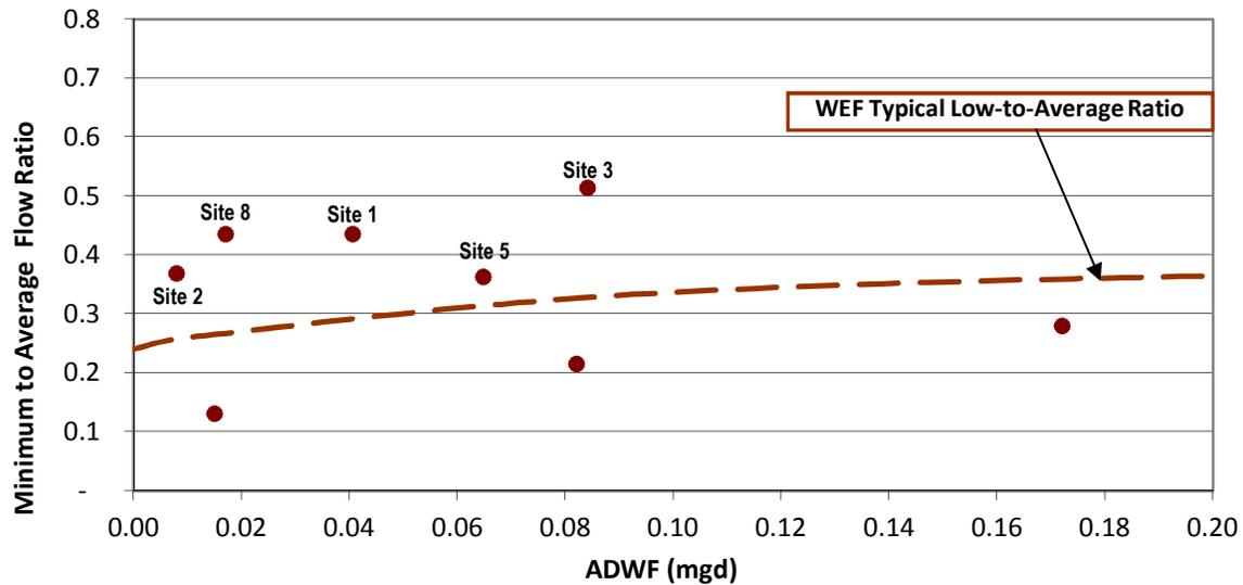
Figure 5-6. Minimum Flow Ratios vs. ADWF<sup>7</sup>
