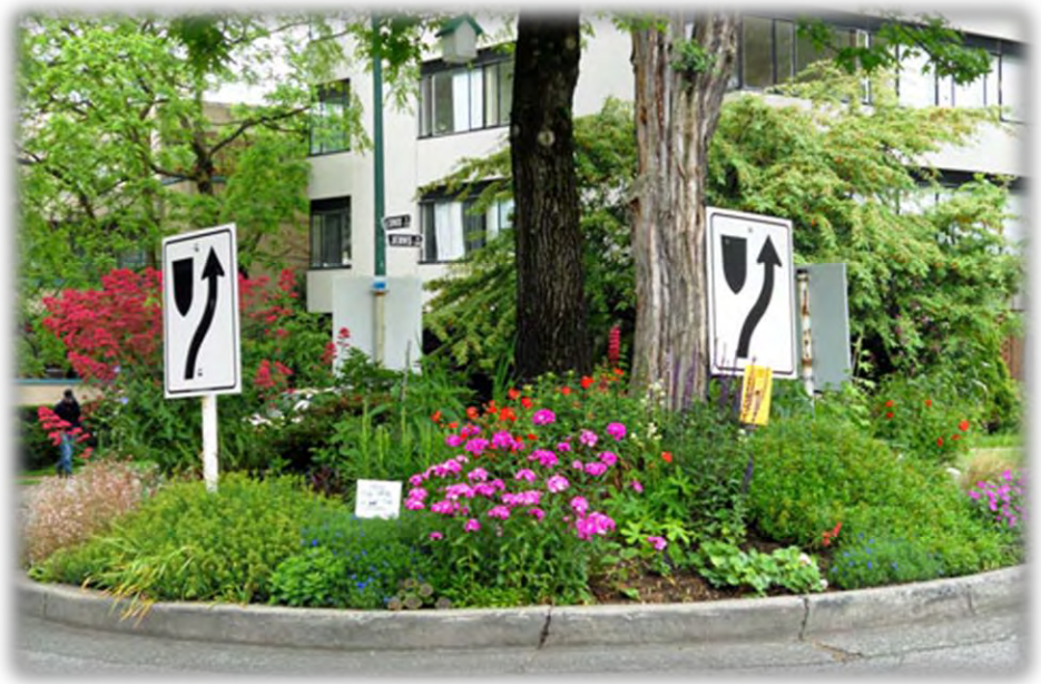
Round-a-bout with raised curb and plantings
