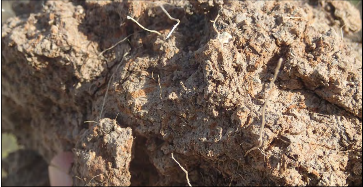
Photograph 5. Representative hydric soil sample at sample point SP4 meeting Redox Dark Surface (F6) hydric soil indicator, and Oxidized Rhizospheres along Living Roots (C3) hydrology indicator.
