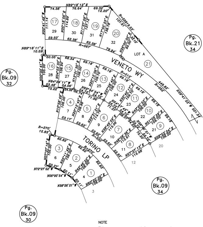
08-06-2014 ALS NOTE Page Redrawn Electronically Formerly POR 021-341-015 & 017 and all of 016-000 All distances on curved lines are length measurements.
