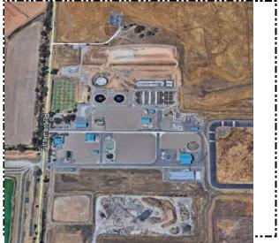
Expand WWTRF capacity by 1.2mgd with addition of Oxidation Ditch and related components. Next expansion will include addition of a Clarifier and related components for additional 0.9mgd of capacity. WWTRF is nearing facility capacity and additional capacity is needed to facilitate future development.
