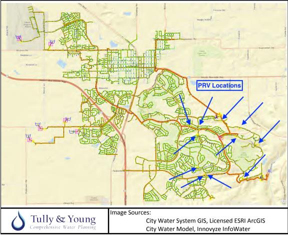
Figure 3-14 – Pressure Reducing Station Locations
