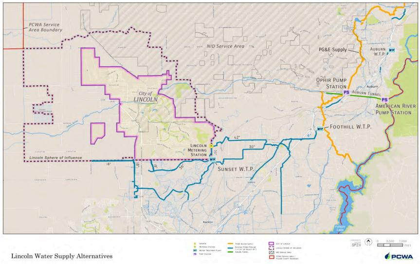
Figure 3-1 – PCWA Existing Transmission Facilities
