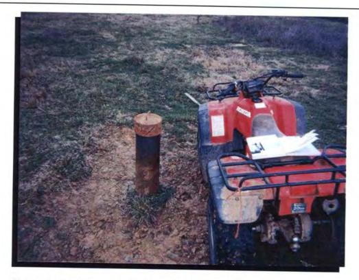
Photo 19: City of Lincoln monitoring well located near the eastern Property boundary on the northern half of the Property.
