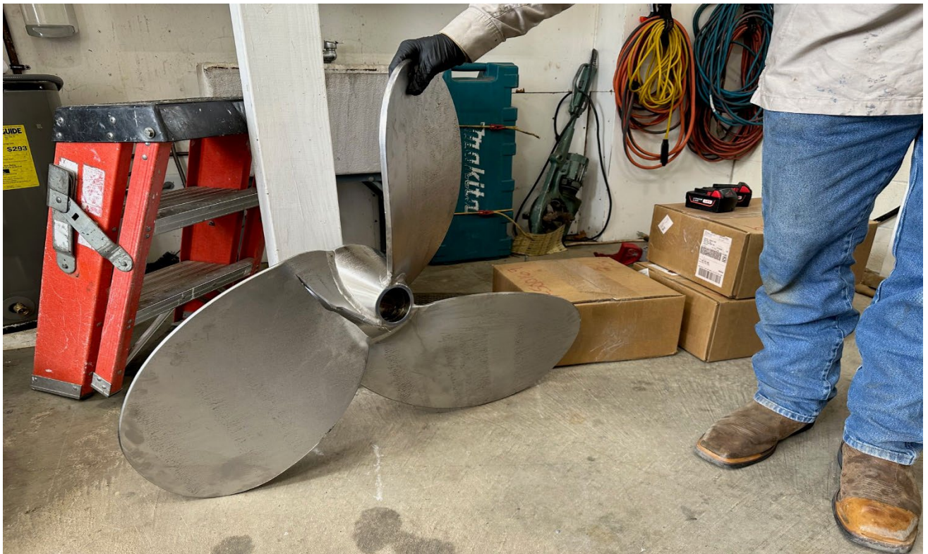
Photo 2. Oxidation Ditch #2, Anoxic Mixer 2B prop damage.
